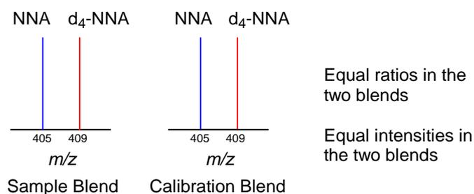
The ratios of analyte to internal standard in each of the sample and calibration solution blends are matched to be equal and the instrumental intensities of all of the analytes are also matched. This technique minimises many of the systematic biases involved in high-accuracy MS measurements.
